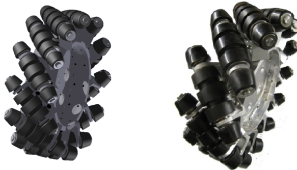
Figure 3: Mecanum Wheels CAD Design [left] Final Product [right]
